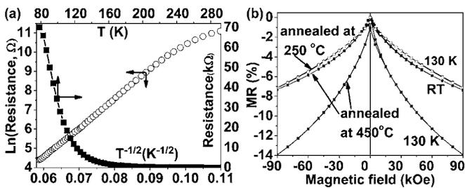
FIG. 4. Nanocomposite with a 65 wt % particle loading: (a) resistance as a function of temperature after heat treatment at  $450^\circ\text{C}$ , and (b) MR vs applied field at room temperature and 130 K.
