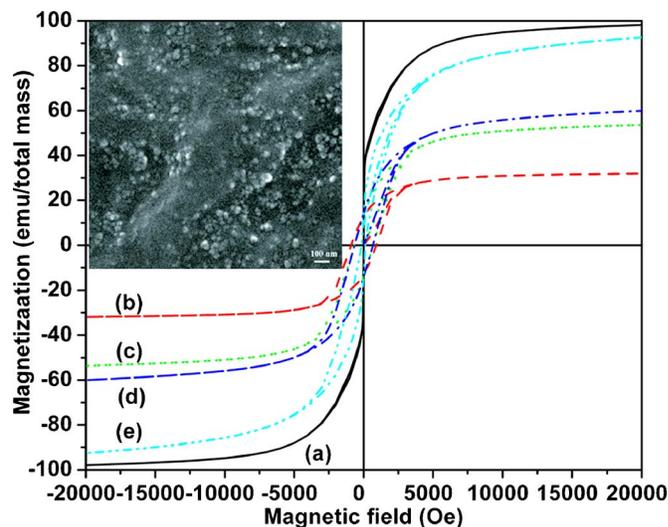
FIG. 3. (Color online) Hysteresis loops of (a) as-received NPs; nanocomposites with a particle loading of (b) 35 wt % and (c) 65 wt %; and nanocomposite with 65 wt % particle loading with heat treatment at (d) 250 °C for 2 h and (e) 450 °C for additional 2 h. The inset shows the SEM image of nanocomposite with a 65 wt % particle loading.
